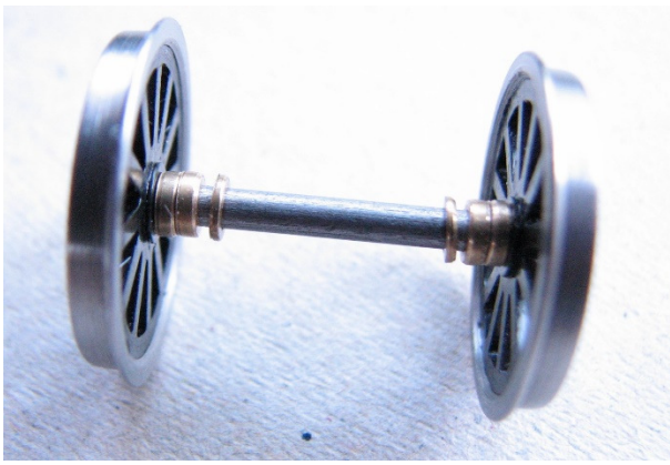
Tender wheels assembled with spacer washers.
