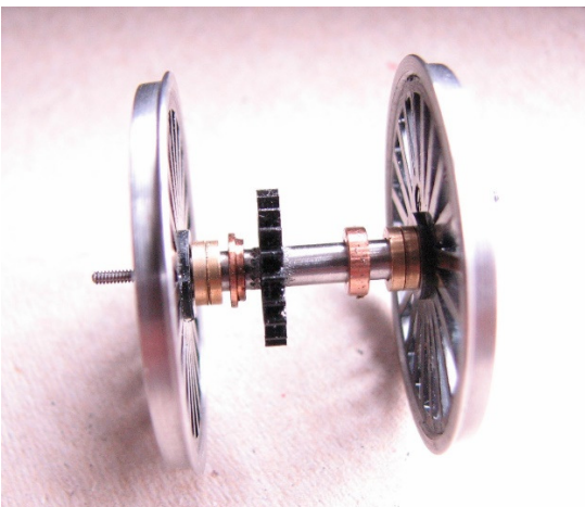
The driven axle with spacing washers and Hornby bushes.
