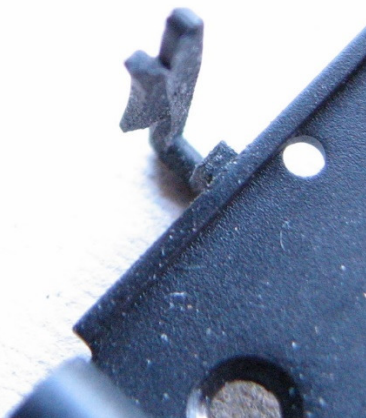
Brake shoes chamfered for clearance.
