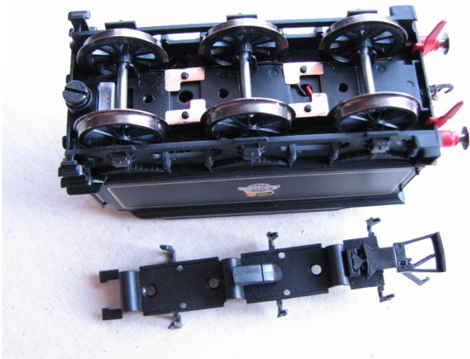
Keeper plate removed – Hornby wheels
